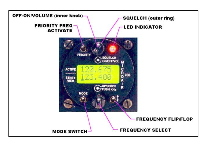
OFF-ON/VOLUME Control: Turn fully anti-clockwise to switch off. Turn clockwise to switch on and adjust volume up.
