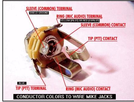
each. Plan ahead and have both wires soldered in place before you put heat shrink over the finished joints. It's okay to have plenty of "unshielded" wire at each microphone jack . . . 2 to 3 inch pigtails hanging out from under the shield will facilitate wiring and will not adversely affect performance.
